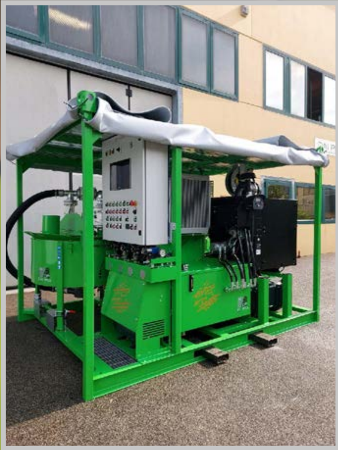
Automatic mixing plant, supplied by silos. They are located at the base of the dam.
